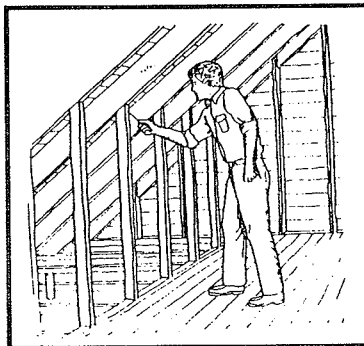
Inspection for termites.
